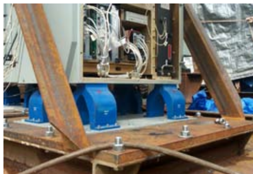
Figure 2 - Elastomer Arch Mounts - base isolation Courtesy Shocktech Inc. and 901D LLC.
