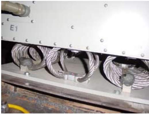
Figure 3 - Cable Isolators - base isolation Courtesy Shocktech Inc. and 901D LLC.
