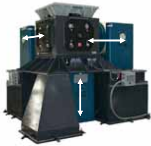
Figure 16-8E Three-shaker Navy 3DoF realization
