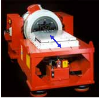
Figure 15-13 Shaker drives Slip Plate
