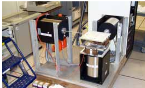
Figure 16-9 Three-shaker 3DoF concept
