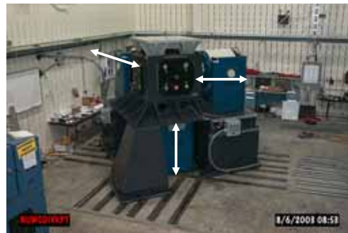
Figure 16-8D Three-shaker Navy 3DoF realization
