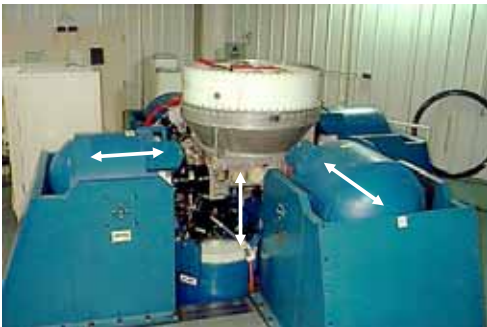
Figure 16-10 USAF Multi-Axis Test Equipment
